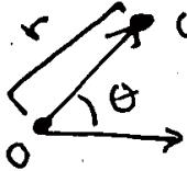
Here we have a fixed axis ray emanating from origin O, and we reach a point  $(r, \theta)$  by making an angle of  $\theta$  radians and goint out a distance of  $r$ .
